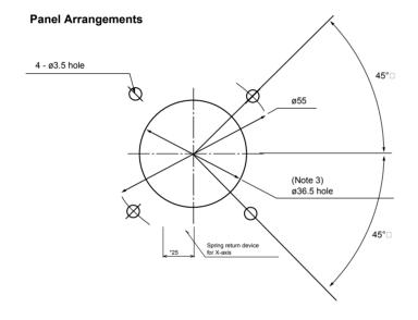
Note: In case of a dust-proof rubber cover is mounted, it is ø44 hole.
