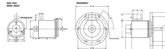
\* AVAILABLE SHAFT DIAMETERS 8 mm - 10 mm (length 20 mm)
