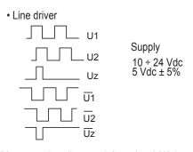
With connection diagram 1-3-4: signal U2 lags signal U1 with clockwise rotation (seen from the shaft side). With connection diagram 2: signal U2 lags signal U1 with anticlockwise rotation (seen from the shaft side).
